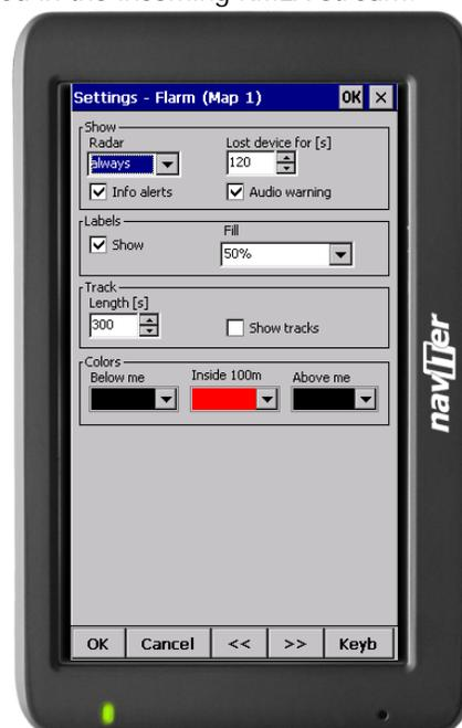
**Show Radar:** Through this setting you may setup a Zoom level below which the Flarm radar is visible. Default value is 10km which is also a suggested value. The reach of the Flarm Radar is about 3km and it depends largely on the placing of the Flarm antenna in both transmitting and receiving aircrafts. The 3km radar circle at Zooms above 10km becomes small and the screen cluttered, therefore we suggest 10km as a default for this setting.
