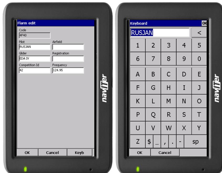
Close all dialogs with OK and you will see an additional line in the Flarm-Radar screen which will report Flarm's friendly name in addition to altitude and vario (see the first screenshot for Friend and Enemy flarms). Additionally when you exit SeeYou Mobile these friendly names will be stored on your PDA for the future. It is a simple text file, so feel free to share it with friends.
