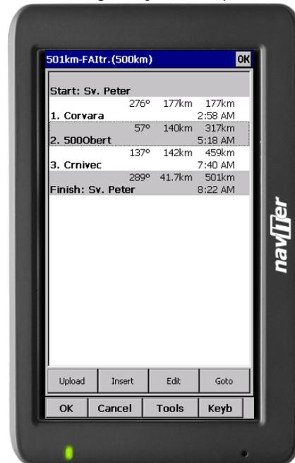
After you have entered the task waypoints, you must setup the properties for the Assigned Areas. Click on the Edit button of each waypoint to open [Edit point](#) dialog. To make the sector an Assigned Area, you should:
