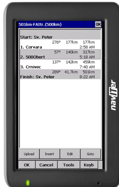
After you have entered the task waypoints, check that waypoint sectors are setup correctly. At each of the waypoints, click on the Edit button to open [Edit point](#) dialog. Setup these values to fly FAI records or badges:
